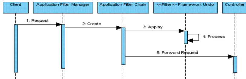
Fig. 5. Sequence Diagram. Undo Framework in Application.
