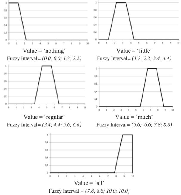
Figure 1. Membership function graphical and fuzzy interval assigned.
